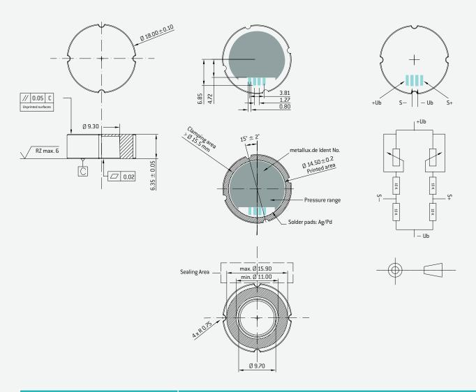
Standard: Tin plated: Sn95.6; Ag3.8; Cu0.6 Type of connection: flat cable
