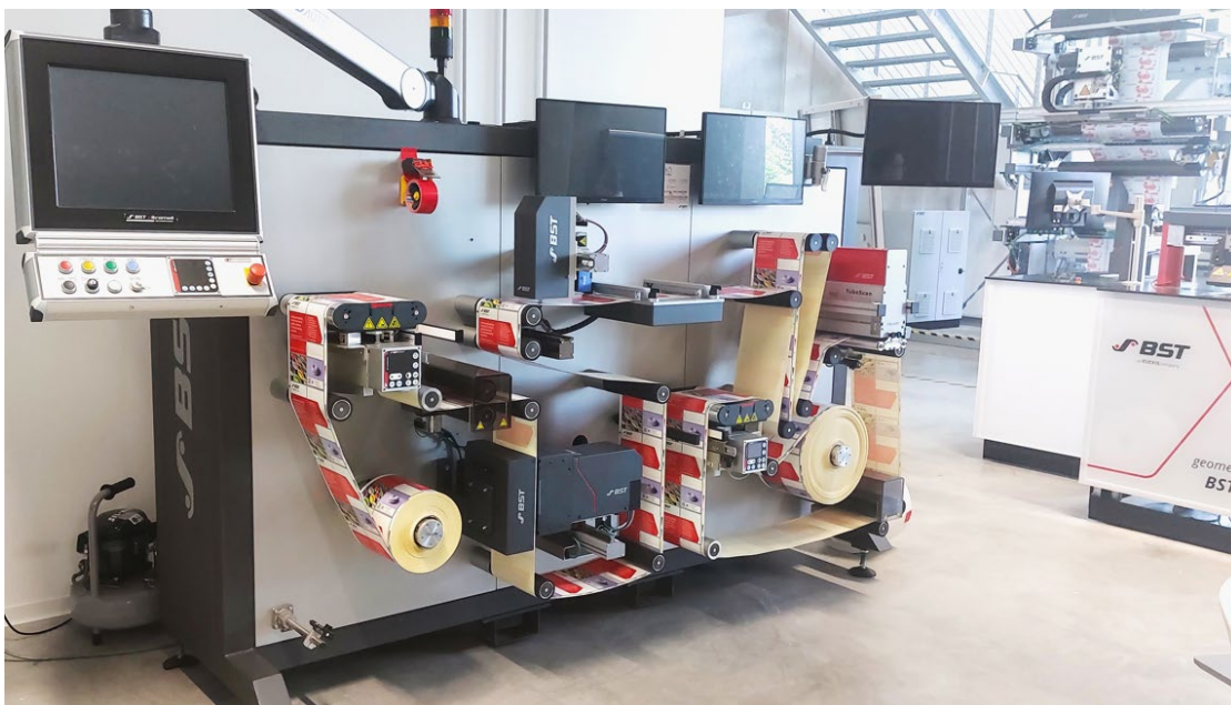
Demo of a web guiding system in the BST showroom in Bielefeld
