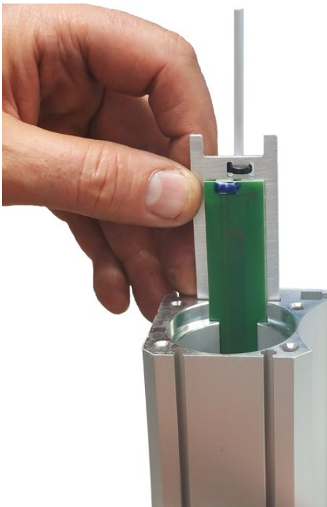
Installation of the sensor in the actuator
